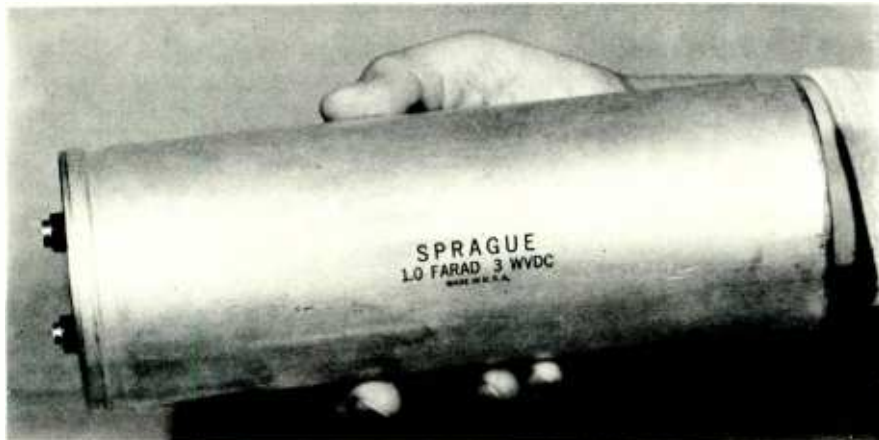
A ONE-FARAD ELECTROLYTIC CAPACITOR provides a whopping amount of filtering and is a mighty handful that you can't expect to find in a transistor radio or recorder.
